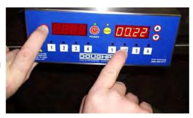
Once you have set the desired time simply press the **TEMP** button, the unit will display the new set-time.
